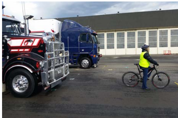
The driver of the truck cannot see the person on the bike.
